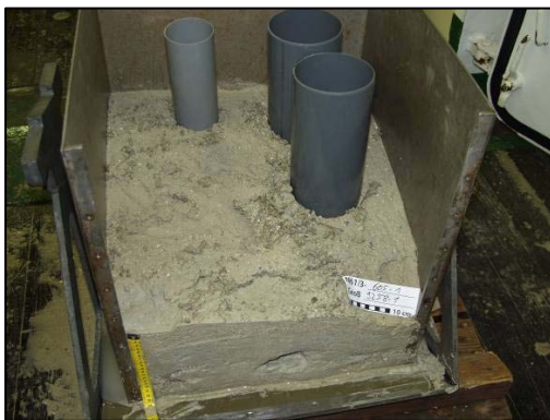
Figure 16. Box corer on the deck. Sediment is collected in the 50cm x 50cm x 50cm “box” in the centre. Note the lid with handle that can be lifted to aid inspection of the retained sediment. The side panels can be removed to allow the sediment vertical profile to be examined and sampled. Source: A.Wheeler
