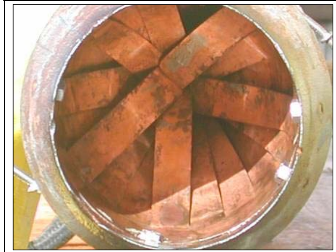
Figure 12. Close up of a core catcher at the end of the barrel stopping recovered sediment from flowing out the end. Source: B.Dorschel
