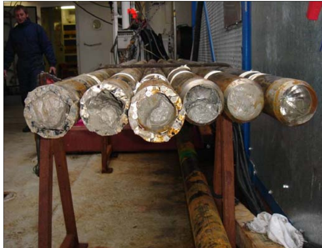
Figure 6. Core ends showing sediment fill. Note: the three of the left were acquired by rotary drilling – note the teeth on the outside of the barrel, the three on the right were from piston coring (see below). Source: A.Wheeler
