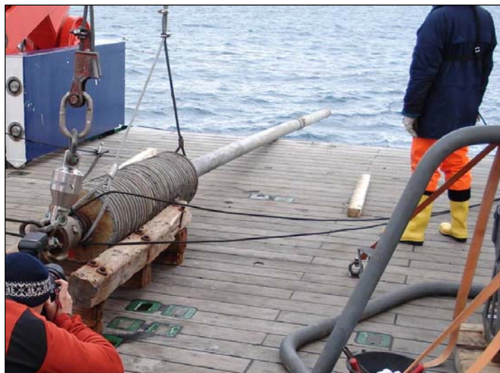
Figure 13. A gravity corer on deck. The maximum length of core is limited by the length of barrel and depth of penetration is limited by the amount of weight on top and resistance of the seabed. Source: B.Dorschel
