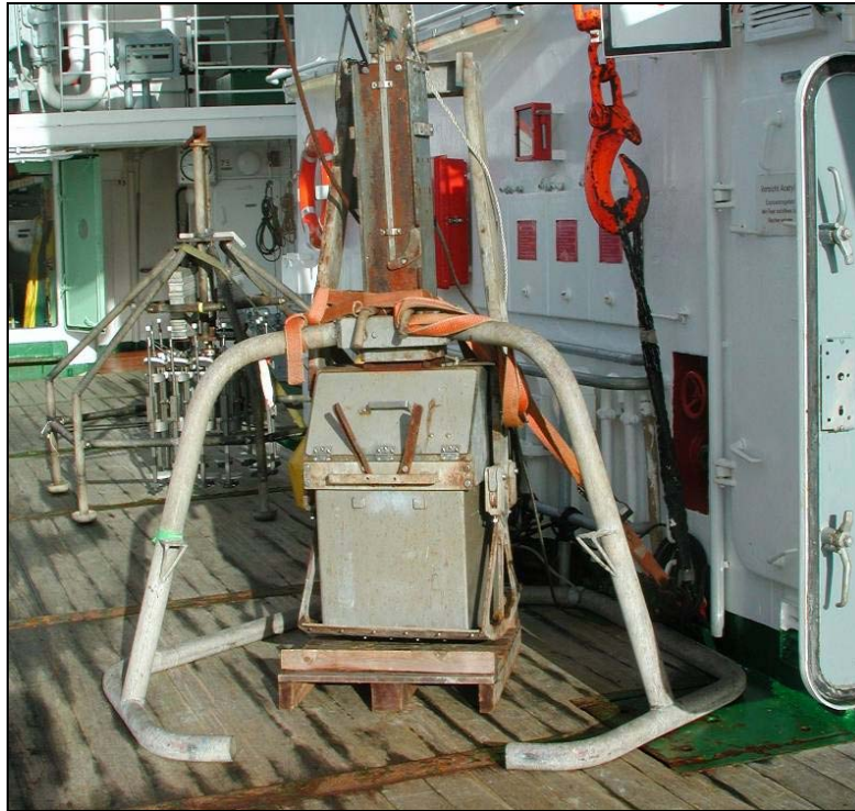
Figure 16. Box corer on the deck. Sediment is collected in the 50cm x 50cm x 50cm “box” in the centre. Note the lid with handle that can be lifted to aid inspection of the retained sediment. The side panels can be removed to allow the sediment vertical profile to be examined and sampled. Source: A.Wheeler
