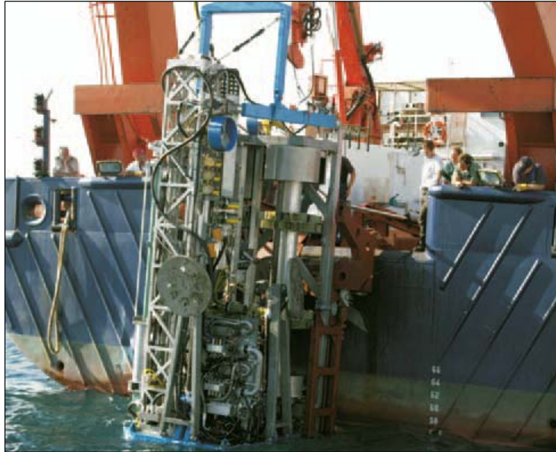
Figure 8. MARUM's drilling rig (MeBo) at the stern of the RV Celtic Explorer. MeBo can be deployed onto the seabed and then drill down 10s of metres. Source: MARUM , Uni. Bremen
