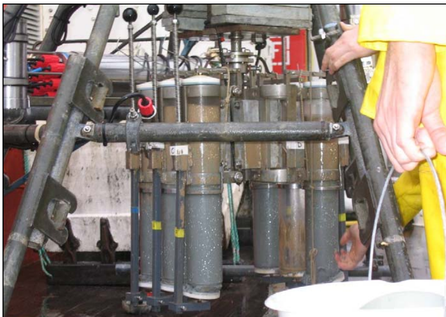
Figure 20. Multicorer showing the sampling tubes filled with sediment and overlying water. Source: A.Wheeler
