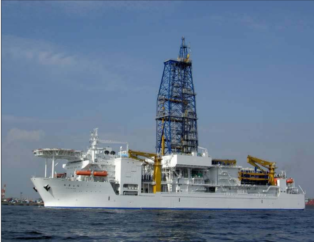
Figure 3. The IODP drillship Chikyu , capable of drilling into the seabed (sediment and rock) to a depth 7 kilometres with near-full core recovery. Source: http://subseaworldnews.com/wp-content/uploads/2012/03/Japan-JAMSTECs-Chikyu-Vessel-Set-Sail-for-IODP-Expedition.jpg
