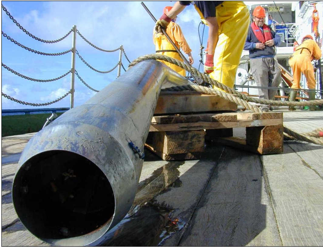
Figure 14. A bent piston core barrel cause by deployment on inappropriate substrates. The so-called “banana-core”. Source: B.Dorschel
