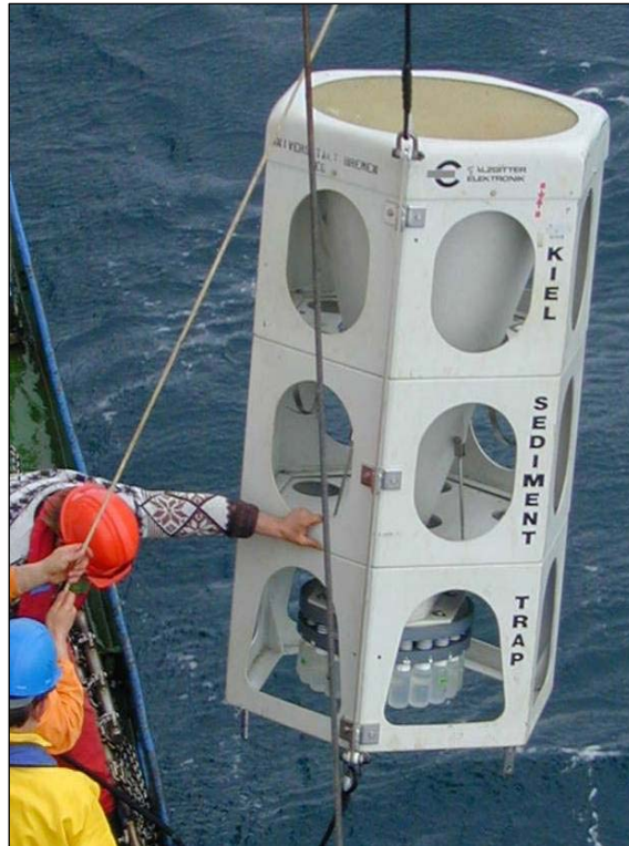
Figure 27. A sediment trap. Note the large funnel at the top and the carousel of sampling bottles at the base. This device will sample sediment falling out of suspension onto the seabed over the deploy interval. The sample bottle carousel can move on at programmable intervals to enable the collection of samples at specified intervals e.g. per tidal cycle.
