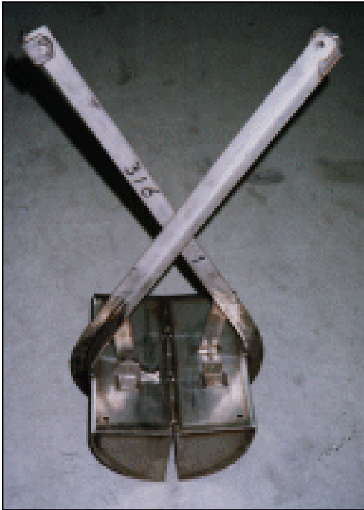
Figure 22. Van veen and hydraulic grab: two examples of the variety of similar grab samplers.
