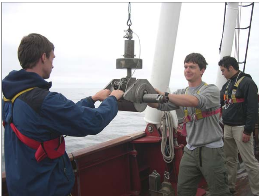
Figure 23. Shipek grab being recovered on deck. The closed drum underneath contains the sediment sample.
