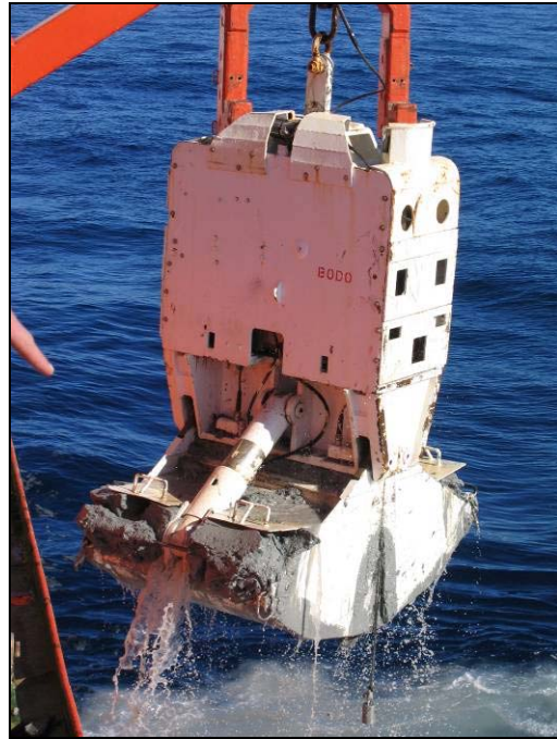
Figure 22. Van veen and hydraulic grab: two examples of the variety of similar grab samplers.
