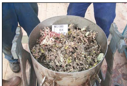
Figure 17. Opened box-core samples and a special circular box-corer called a Reineck corer. Source: B.Dorschel
